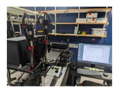
**Bio-Imaging (BIRC):** The Nikon Ring TIRF was fully commissioned and is already highly popular. The new custom-built SCAPE (Swept Confocally-Aligned Planar Excitation) system is available in the Beckman Advanced Center for Light-sheet Microscopy (BALM). The SCAPE allows high-speed volumetric imaging of living samples, including moving organisms (currently limited to 20x magnification).
